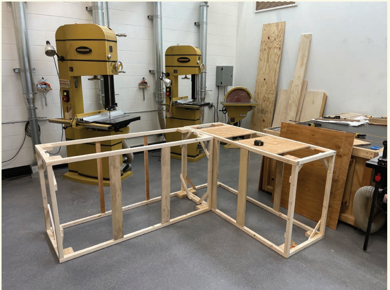
Internal support structure made from 2x2 lumber and recycled shipping crates
