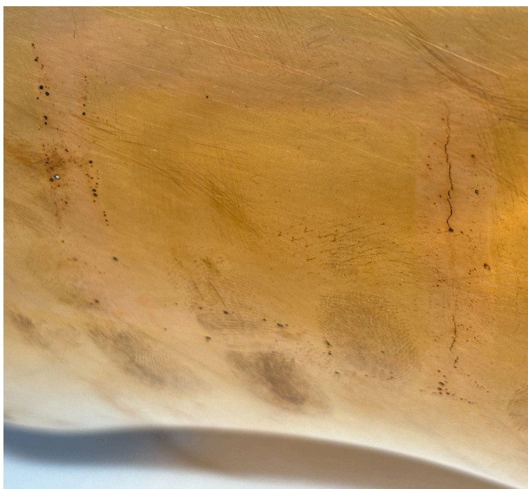
Figure 1. Microfissure and surface pitting.
