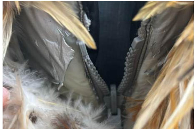
Figure 16. Delamination of the metallic coating, front collar.
