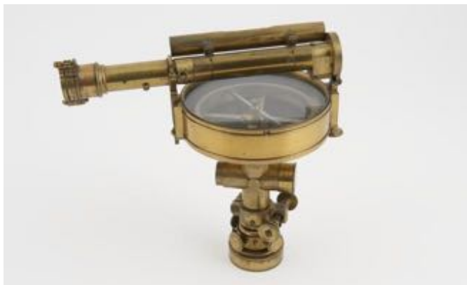
Figure 8. Improved Patent Portable Theodolite, consisting of prismatic compass, telescopic sight and level by C. A. Schmalcalder, 82 Strand, London, England, 1818-1826. Image courtesy Science Museum Group (1911-180).
