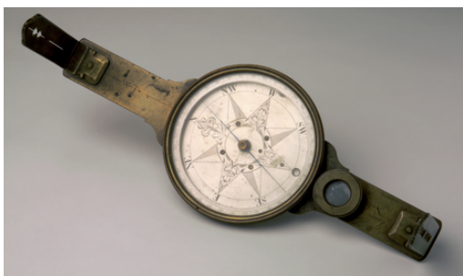
Figure V-1. Surveying compass made by Isaac Chandlee (Chester, PA). 1790-1813. Image courtesy Winterthur Museum (2003.0054).
