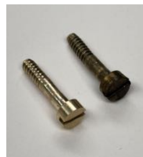
Figure 28. Matched dimensions of the replacement screw.
