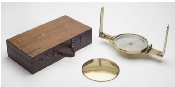
Figure V-3. Surveying Compass, Field Case, and Box made by Frederick Augustus Heisely Jr (Dauphin, PA). 1820-1836. Image courtesy Winterthur Museum (2010.0042.001).
