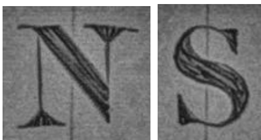
Figure 16. Incised metal of compass dial lettering. Crop of X-radiograph without filter.
