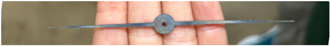
Figure 32. Needle, tempered with a torch to around 575°F (300°C), the temperature at which a blue iron oxide layer forms. Image courtesy Mia Kaplan.
