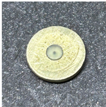
Figure 35. Sapphire flush with the underside of the needle cap. The hole in the center marks the surface where the pivot comes into contact with the needle. The sapphire was provided by Brittany Cox. Image courtesy Mia Kaplan.
