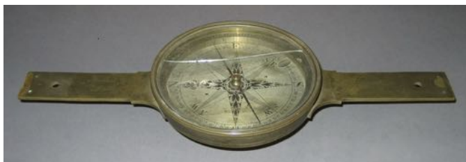
Figure V-5. Surveying compass made by Henry Shuttleworth (London, UK). 1780-1798. Image courtesy Winterthur Museum (1969.2041A).
