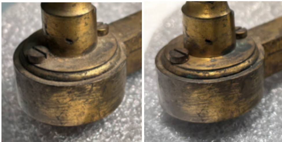
Figure 19. Detail of the south end instrument attachment arm before (left) and after (right) solvent cleaning.
