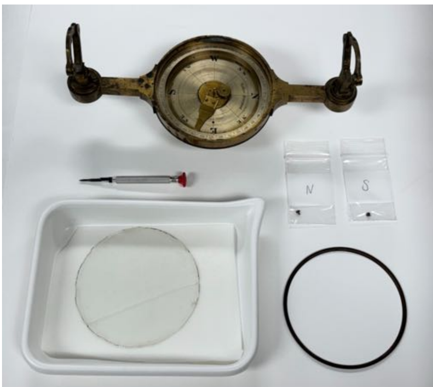
Figure 13. Cover glass removed and components separated.
