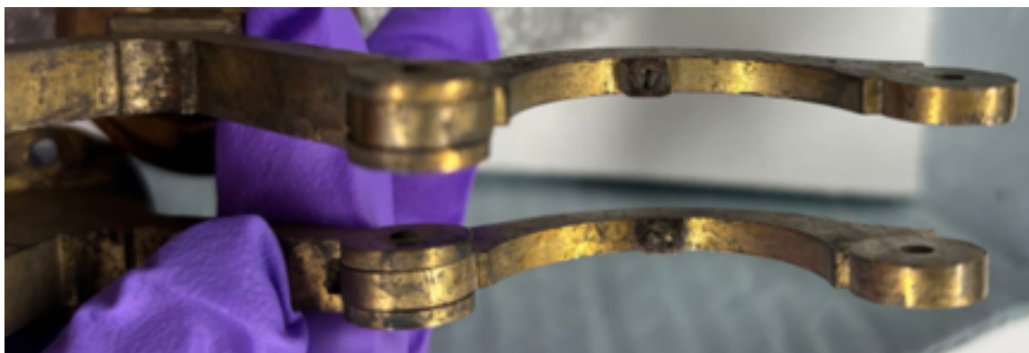
Figure 22. Original instrument holder pad (top) and replacement (bottom).
