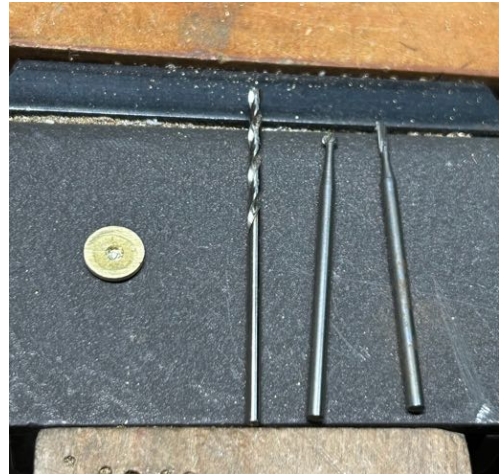
Figure 34. Needle cap, underside hole for jewel bearing. Mia created the hole with the three tools pictured: a drill bit, ball bur, and baby end mill. Image courtesy Mia Kaplan.
