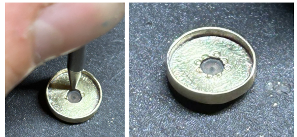
Figure 36. Bead-set sapphire (left image: process; right image: complete), with lip to create a pressure-fit reversible lid attachment between this component and the lathe-turned needle cap. Image courtesy Mia Kaplan.
