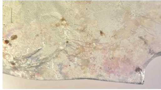
Figure 9. Microcracks near the break edge, fragment 2 exterior, 100x magnification.
