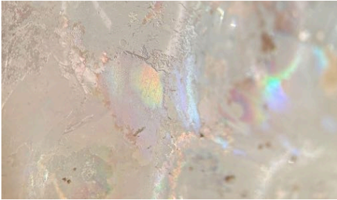
Figure 8. Opalescent weathering, fragment 2 exterior, 100x.
