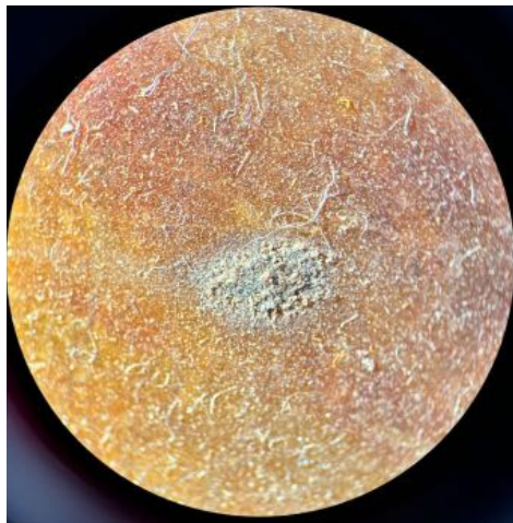
Figure 21. Micrograph of surface accretion on the lower center of the cape. 160x magnification.
