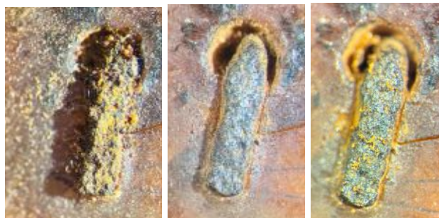
Figure 22. Before (left), immediately after (center), and two weeks after (right) mechanical corrosion reduction.
