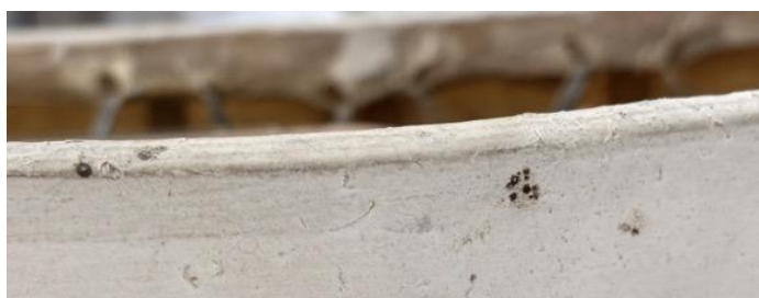
Figure 19. Dark accretions and soiling deposits on the hull exterior.
