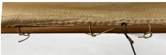
Figure 24. Three of six knots, before tightening threads.
