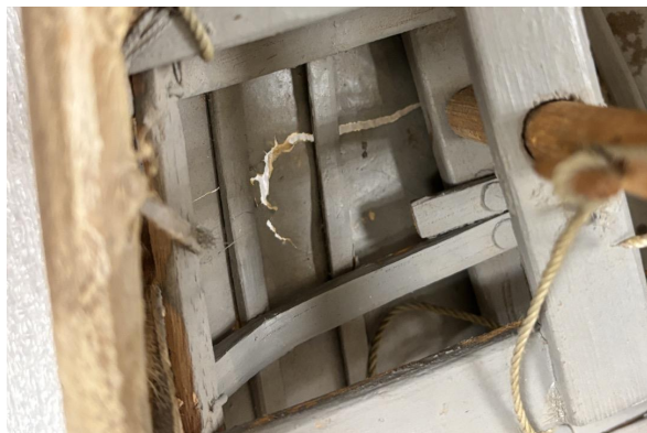
Figure 11. Hull tear (interior, PL bow).
