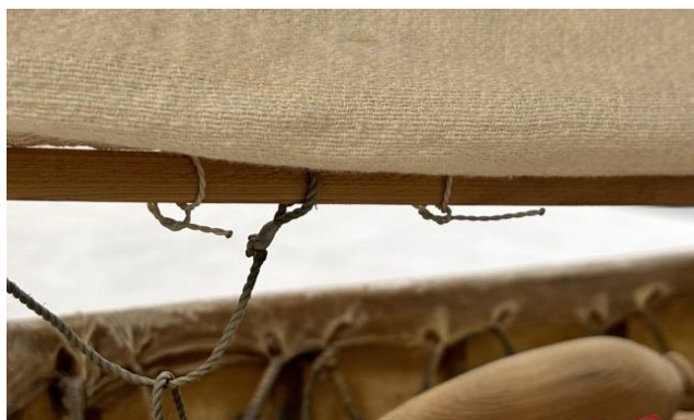
Figure 12. Loose knots that attach the sail to the boom.
