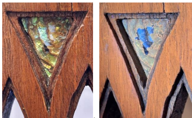
Figure 14. Yellowed coating over the inlay, particularly visible in this area of incomplete coating. Left: visible light. Right: UV (365 nm) uvBeast V3 flashlight.
