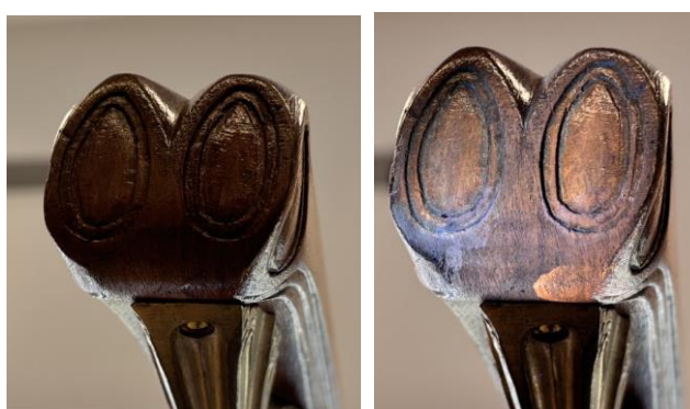
Figure 11. UV evidence of multiple coating applications/removal of prior coatings. Left: visible light. Right: UV (365 nm) uvBeast V3 flashlight.
