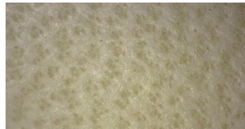
Figure 4. Replacement parchment seat. Captured with a Dinolite Edge and DinoCapture 2.0 software.
