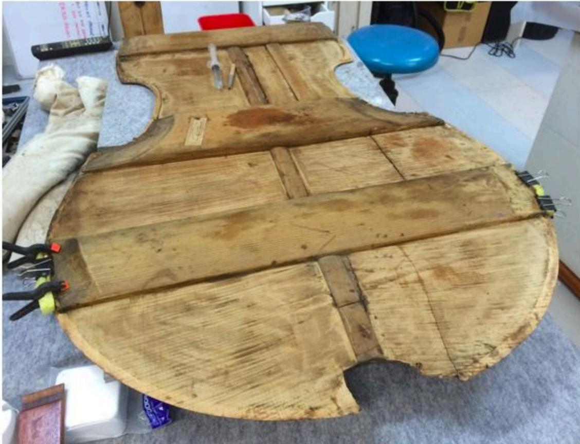
*Typical old ladder-braced back, complete with shrinkage cracks and loose braces*
