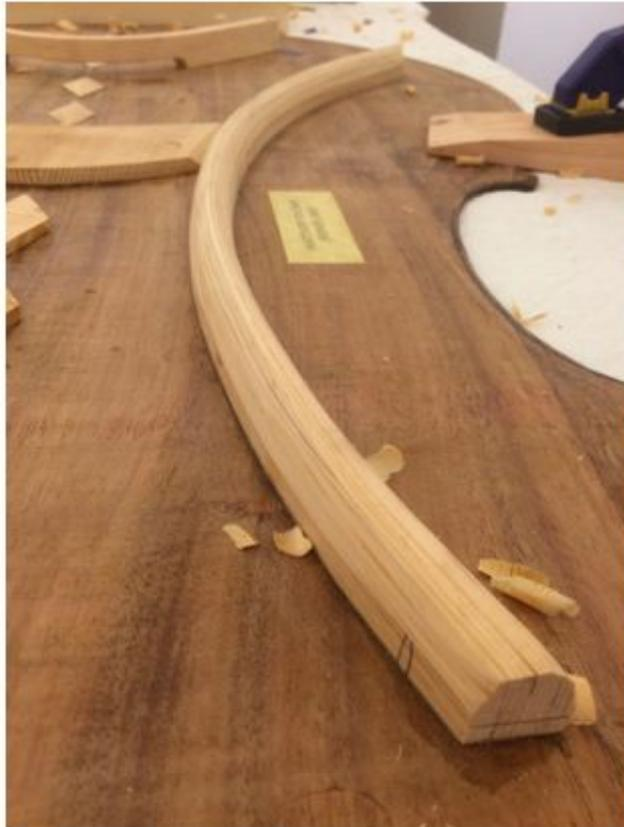
*Detail of brace shaping: ends can be finished in a variety of styles*
