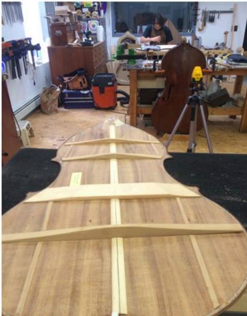
*A new cross-braced top, with split centre seam and a loose lower brace end, caused by one week in a non humidified environment ... a dry New York winter.*
