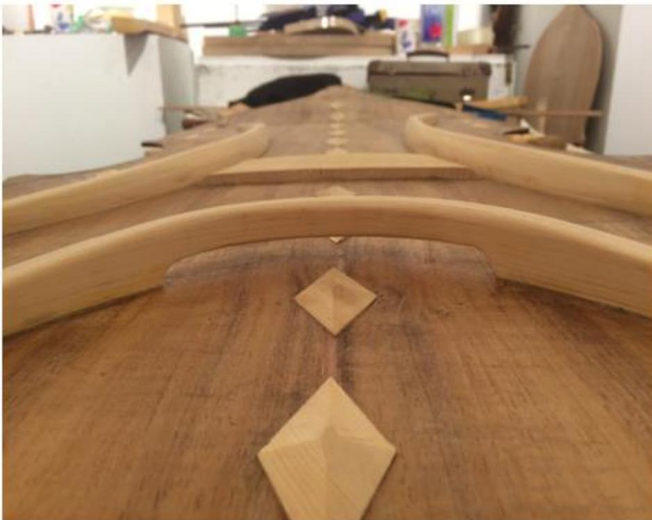
*Detail of brace layout showing the boomerang brace cut-out*
